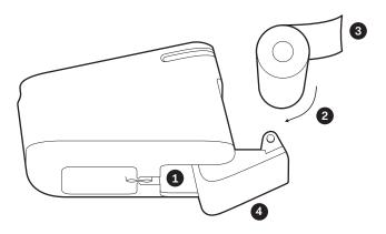
**1.** Press firmly on the bottom side of the paper hatch.
