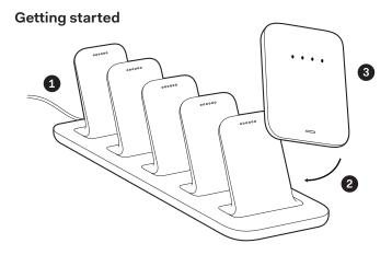
**1.** Connect the USB-C cable to the station and plug it into a power socket using the included adapter (min. 5V and 2.4A).
